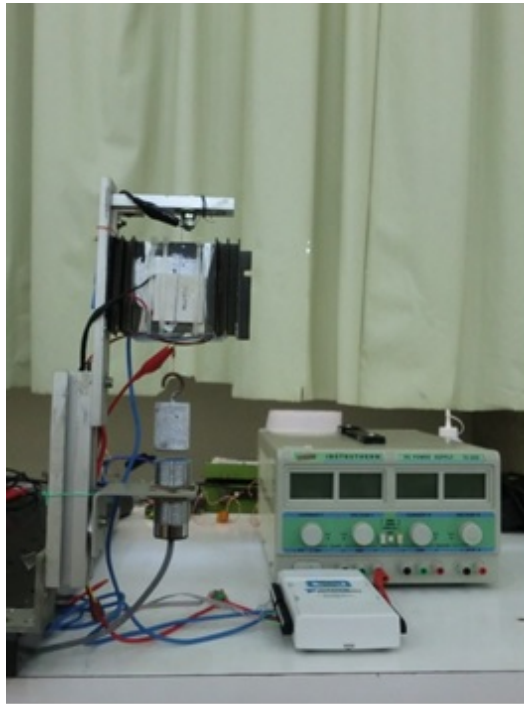
Figure 3.13: Image of the built system for the SMA actuator validation.
