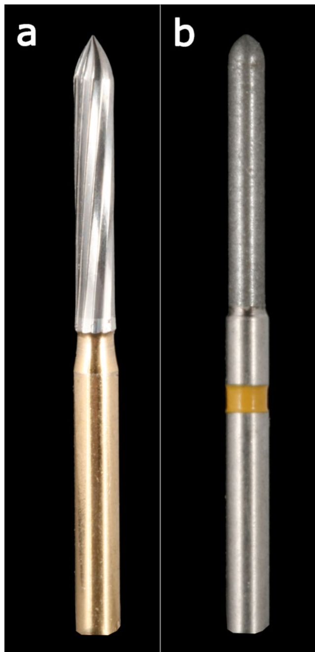
Figure 1. Dental finishing instruments: (a) 30-blade carbide bur and (b) 30- \mu\text{m} finishing diamond bur.
