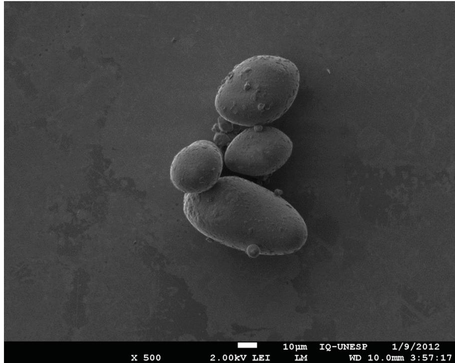
**Figura 27 – Fotomicrografia do HPMCP**
