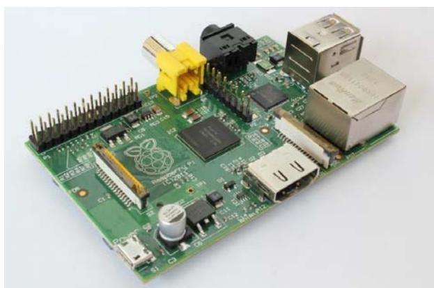
**Figura 2.** Placa *RaspBerryPi* (RAULINO, 2013)
