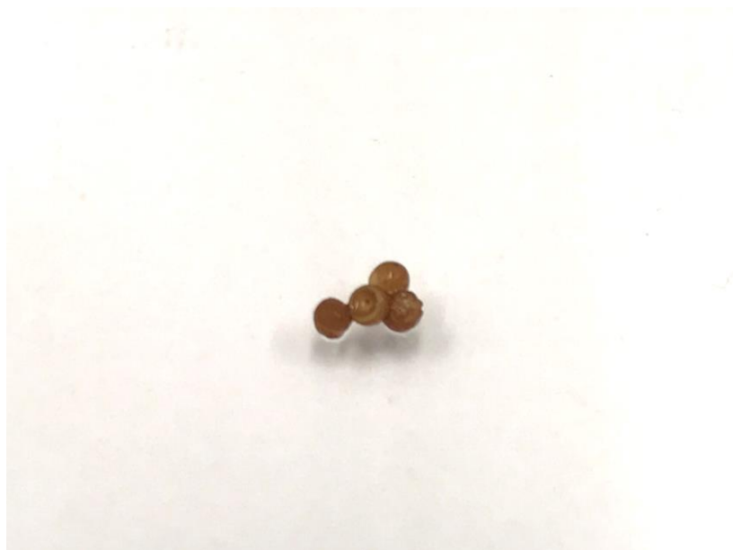
Figure 11 – Chitosan beads resulting after natural organic matter contact
