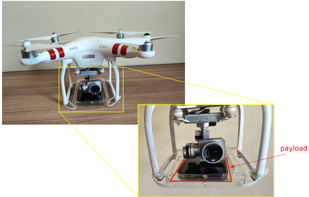
Figure 1 – Experimental set-up for a fixed payload configuration.
