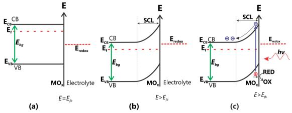
Fig. 2 Band bending when an n-type SC is under a  $E=E_{fb}$ , b  $E>E_{fb}$ , and c  $E>E_{fb}$  and irradiated by light with  $h\nu \ge E_{be}$
