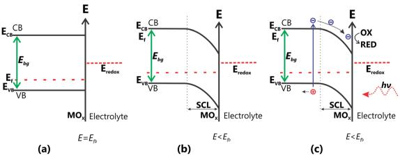
Fig. 5 Band bending when a p-type SC is under a  $E=E_{\rm fb}$ , b  $E<E_{\rm fb}$ , and c  $E<E_{\rm fb}$  and irradiated by light with  $h\nu \ge E_{\rm bg}$
