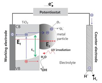
Fig. 7 Schematic depiction of the photoelectrocatalytic mechanism of  ${\rm TiO_2}$  coupled to a metal particle
