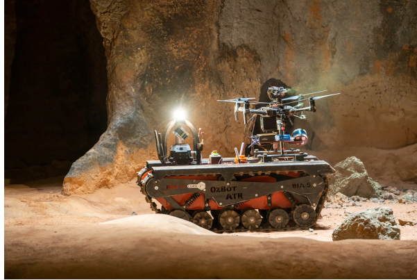
Figure 2.2 – An example of tracked robot. Adapted from https://research.csiro.au/robotics/our-work/darpa-subt-challenge-2018/
