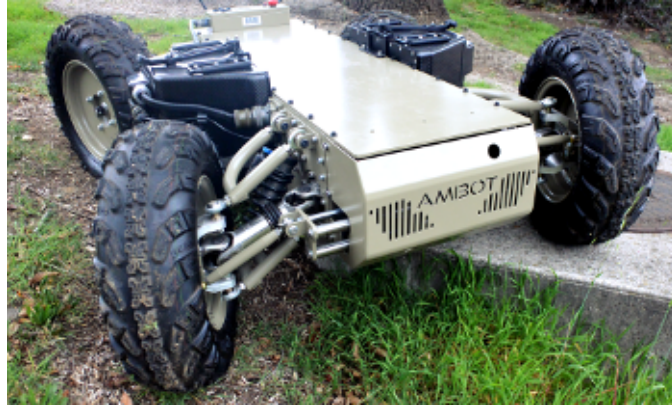
Figure 2.1 – An example of four-wheel independent drive robot. Adapted from http://www.ambot.com/ip-wheel.shtml
