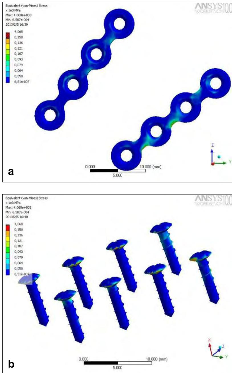
Figure 9. Group Eng 2P: von Mises equivalent stress ( $\sigma_M$ ) for the (a) plates and (b) the screws.
