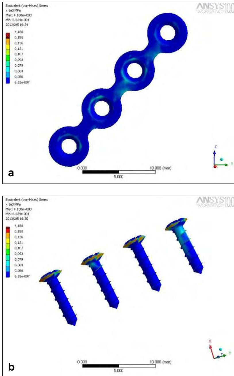
Figure 8. Group Ti-15Mo 1P: von Mises equivalent stress ( $\sigma_M$ ) for the (a) plate and (b) the screws.
