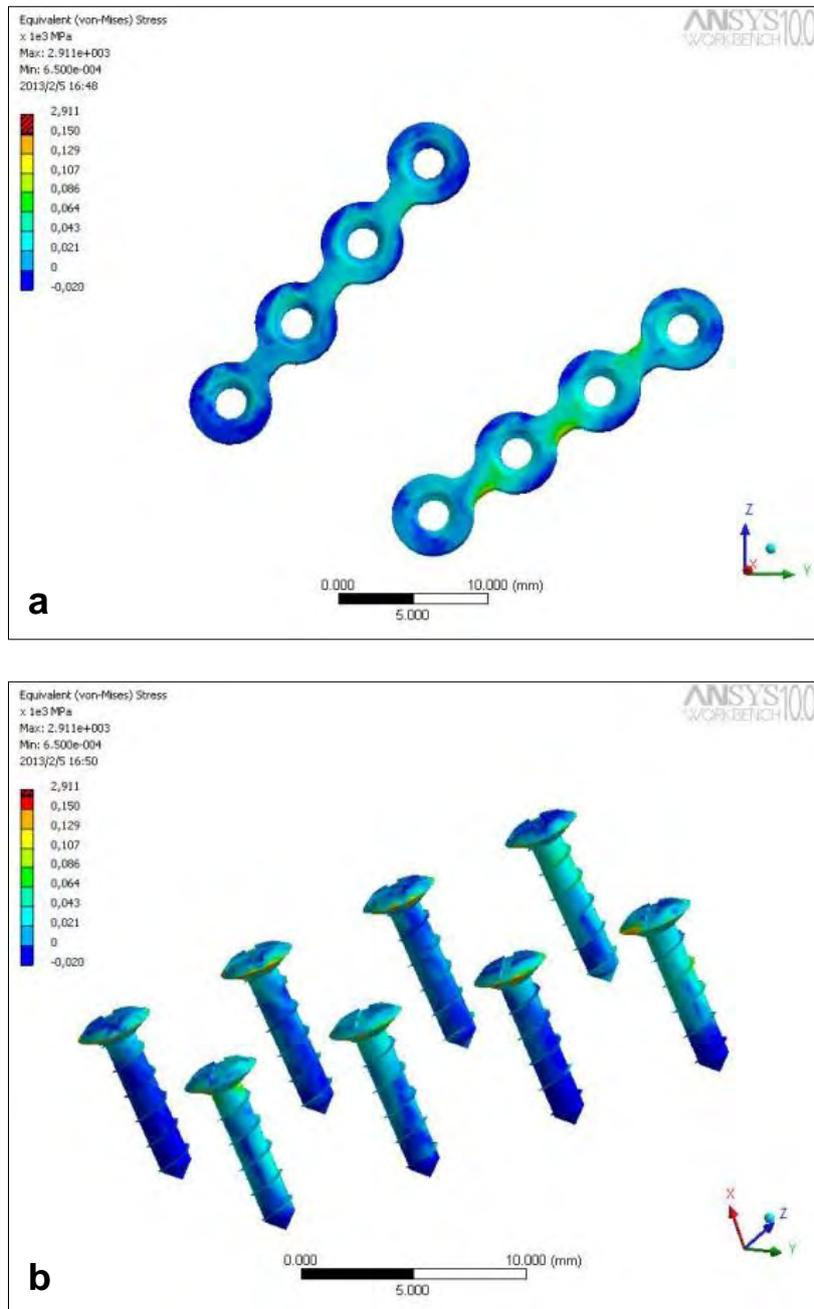
Figure 10. Group Ti-15Mo 2P: von Mises equivalent stress ( $\sigma_M$ ) for the (a) plates and (b) the screws.
