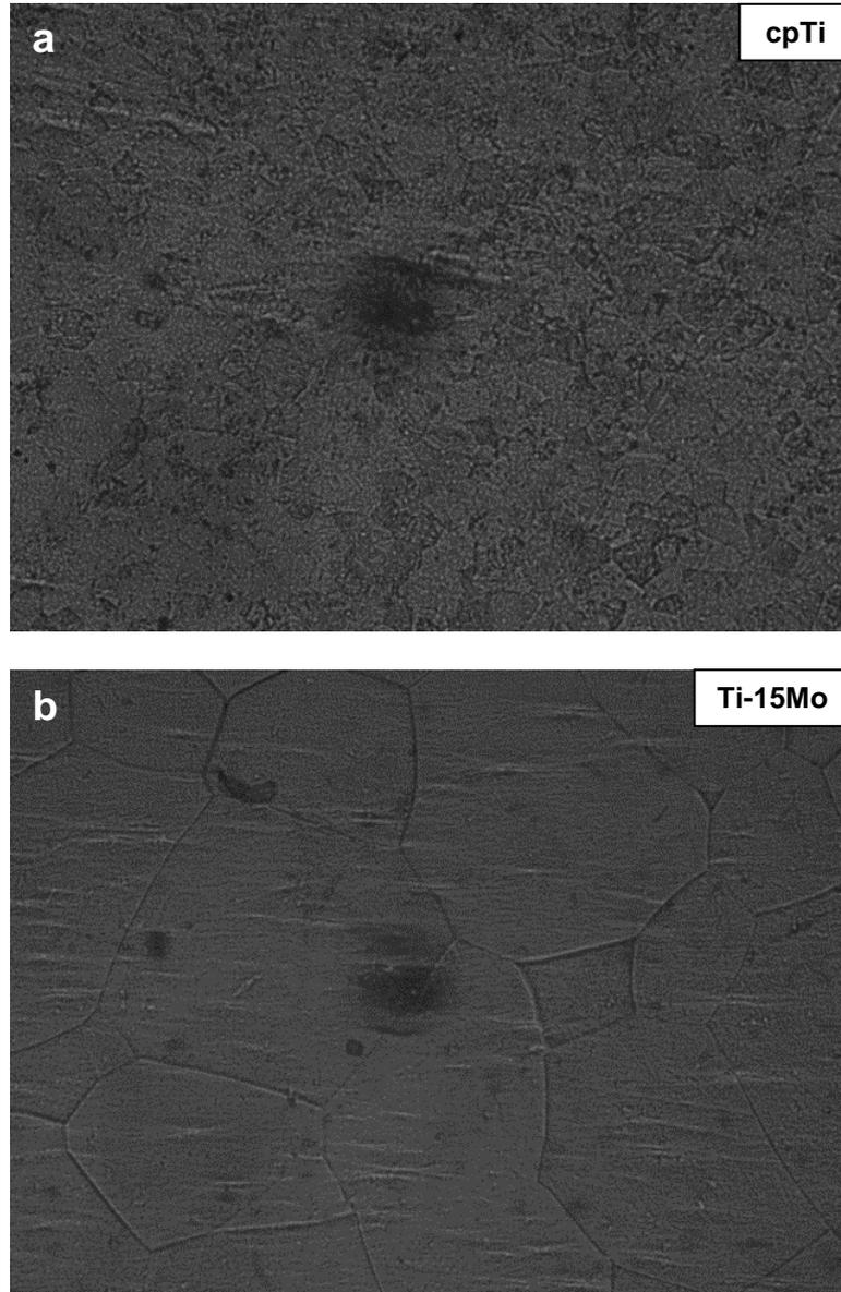
Figure 5. Optical microscopy of the plates, after the surface attack with Kroll solution, revealing the microstructures of the (a) cpTi and the (b) Ti-15Mo alloy.
