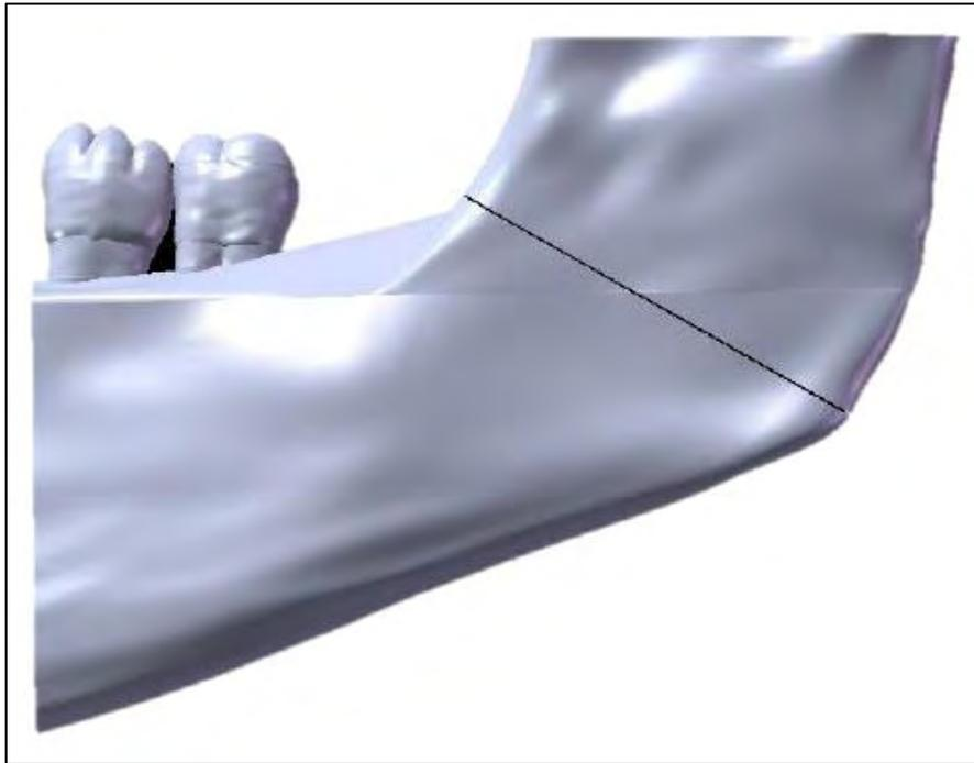
Figure 3. Reconstruction of the mandible segment (SolidWorks 2010) simulating the fracture in the mandibular angle.
