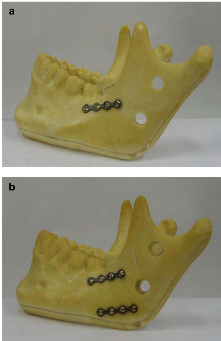
Figure 1. The location of the titanium-based system for both internal fixation techniques, (a) 1 plate and (b) 2 plates.
