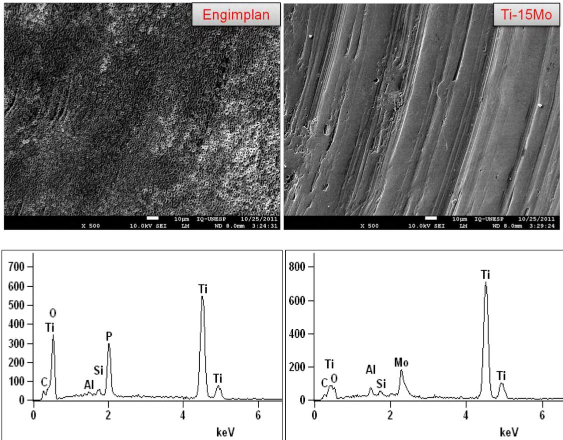
Figure 7. (top) SEM micrograph showing the plates (Engimplan e Ti-15Mo) morphology (plate thread); (bottom) EDX of the same surfaces. Magnification 500X.
