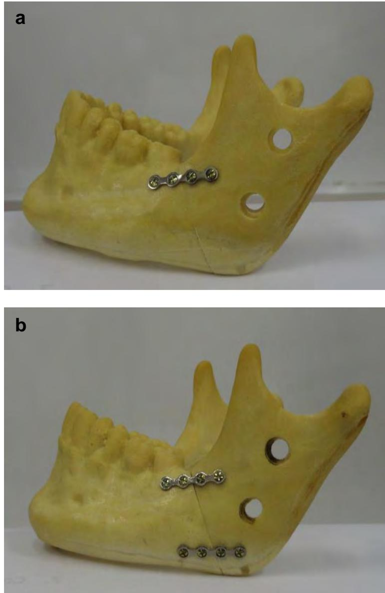
Figure 2. The location of the titanium-molybdenum-based system for both internal fixation techniques, (a) 1 plate and (b) 2 plates.
