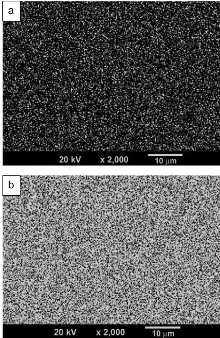
Figure 4. SEM micrograph of Ti-15Mo alloy sample; (a) Mo mapping (white points) and (b) Ti mapping (white points) of the Ti-15Mo alloy sample.
