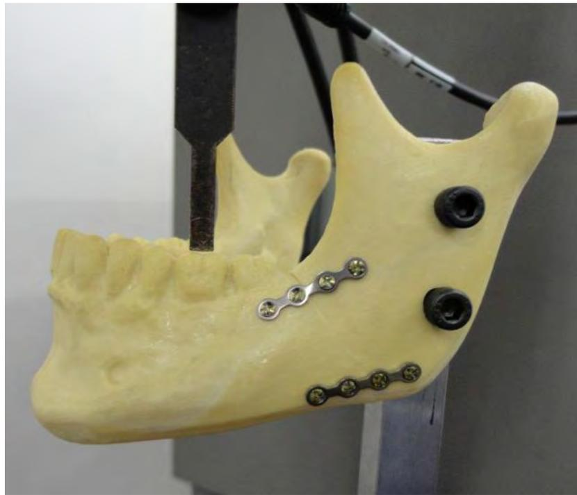
Figure 3. Vertical linear load applied at the first inferior molar, during the mechanical test on a servo-hydraulic machine.
