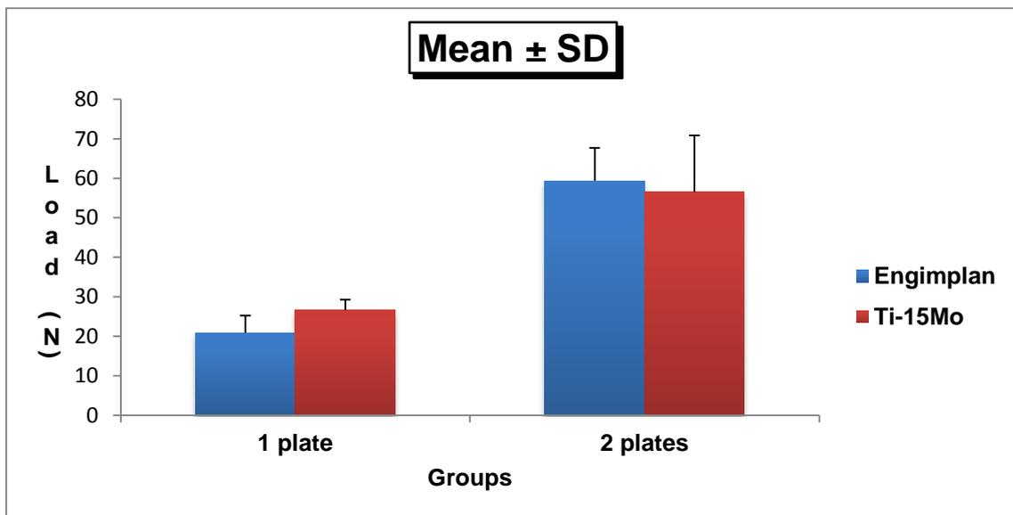
Figure 8. Mean and standard deviation (SD) of the results obtained in the biomechanical analysis, considering the material of the bone plates and the internal fixation technique employed (two-factor factorial ANOVA).
