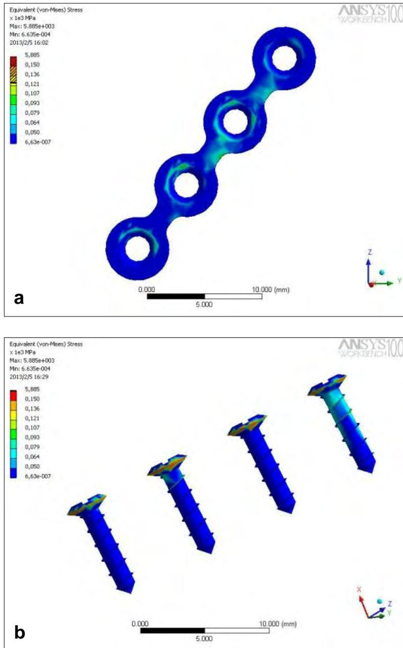
Figure 7. Group Eng 1P: von Mises equivalent stress ( $\sigma_{vM}$ ) for the (a) plate and (b) the screws.
