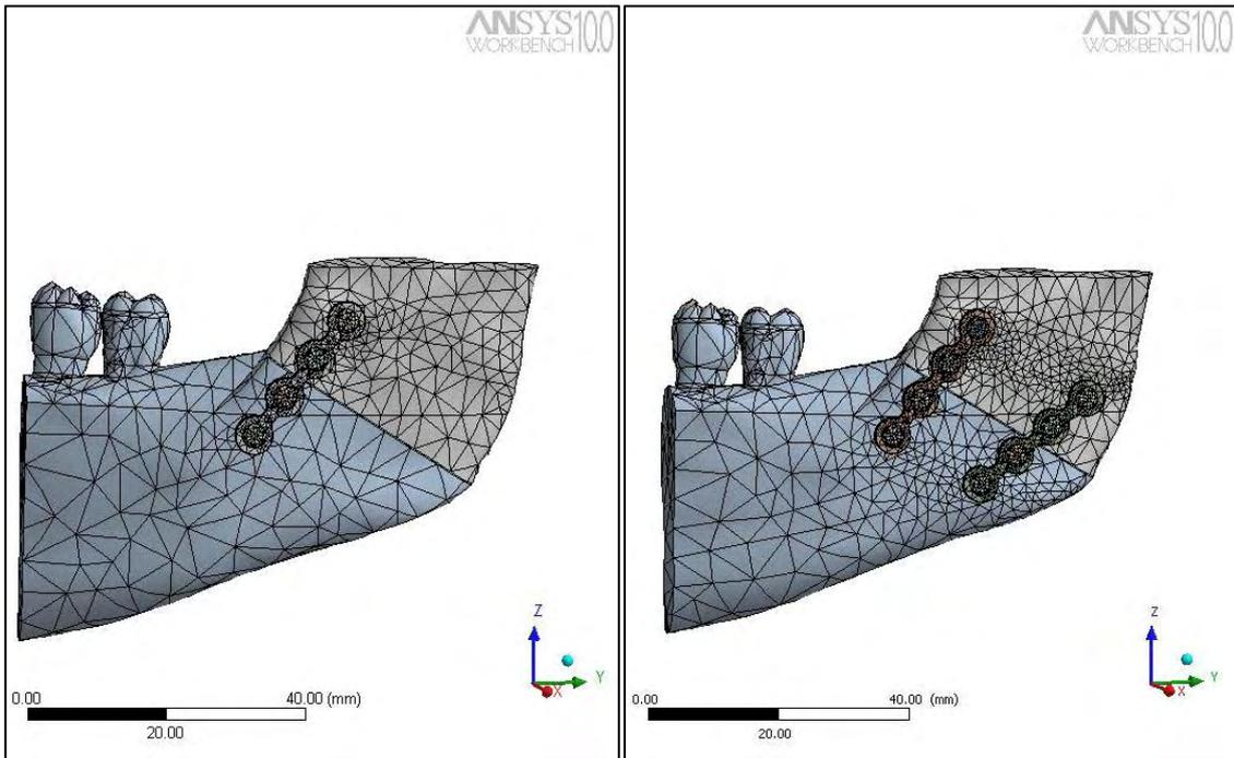
Figure 5. Meshed models showing the 2 plate configurations analyzed in the study: (left) 4-hole monocortical tension band plate at the superior border, and (right) 4-hole monocortical tension band plate and 4-hole bicortical compression band plate at the inferior border.
