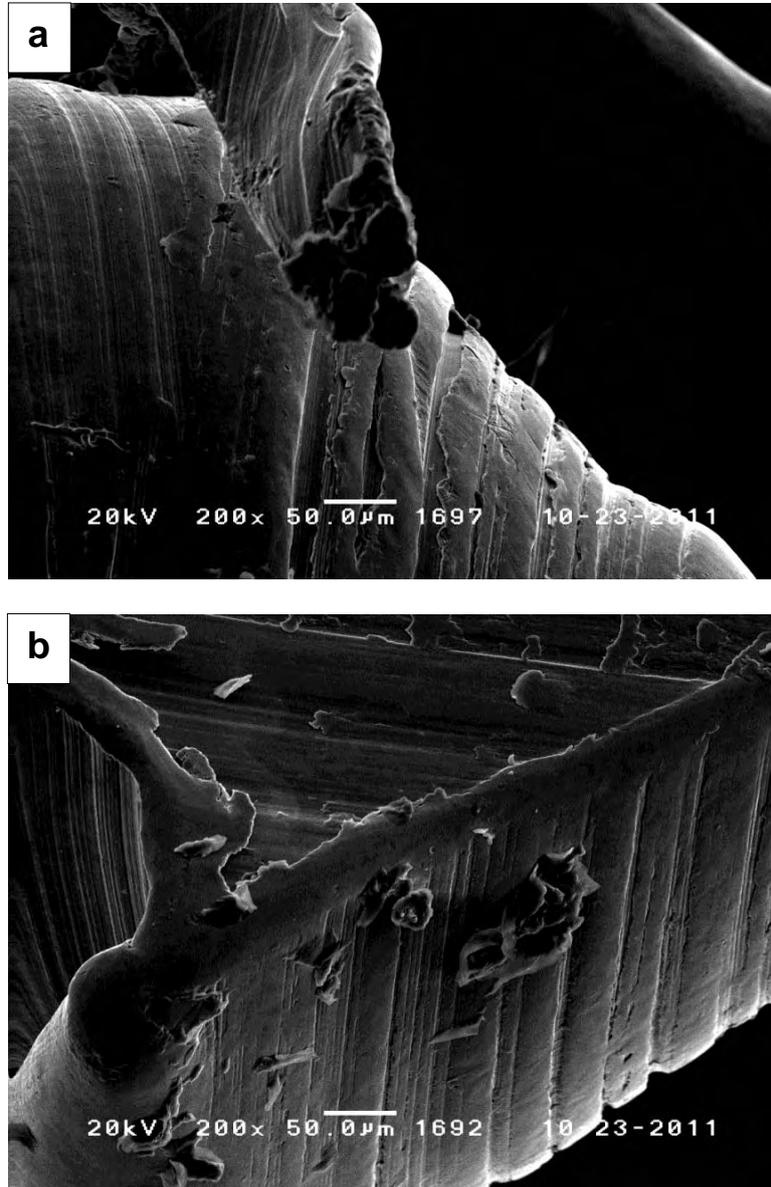
Figure 6. SEM micrograph showing the screw (Ti-6Al-4V) morphology; (a) screw tip and (b) screw thread. Magnification 200X.
