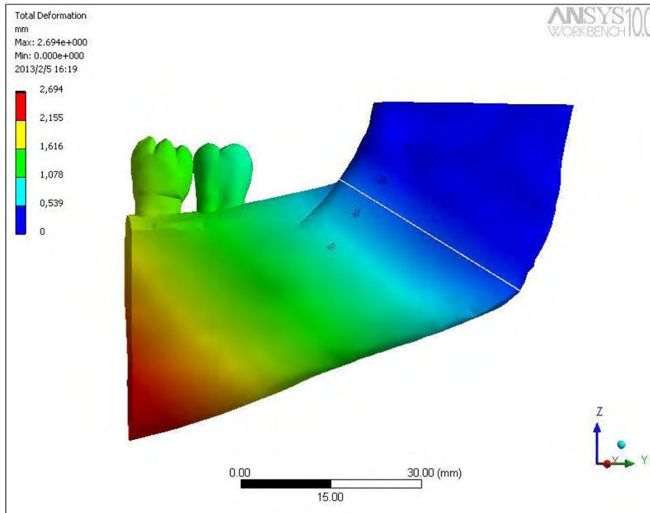
Figure 6. Stress distributions in the mandibular model by a 100 N vertical load.
