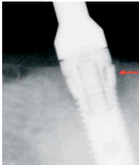
Fig. 5. Digital periapical radiography of tilted implant fractured at platform level.
