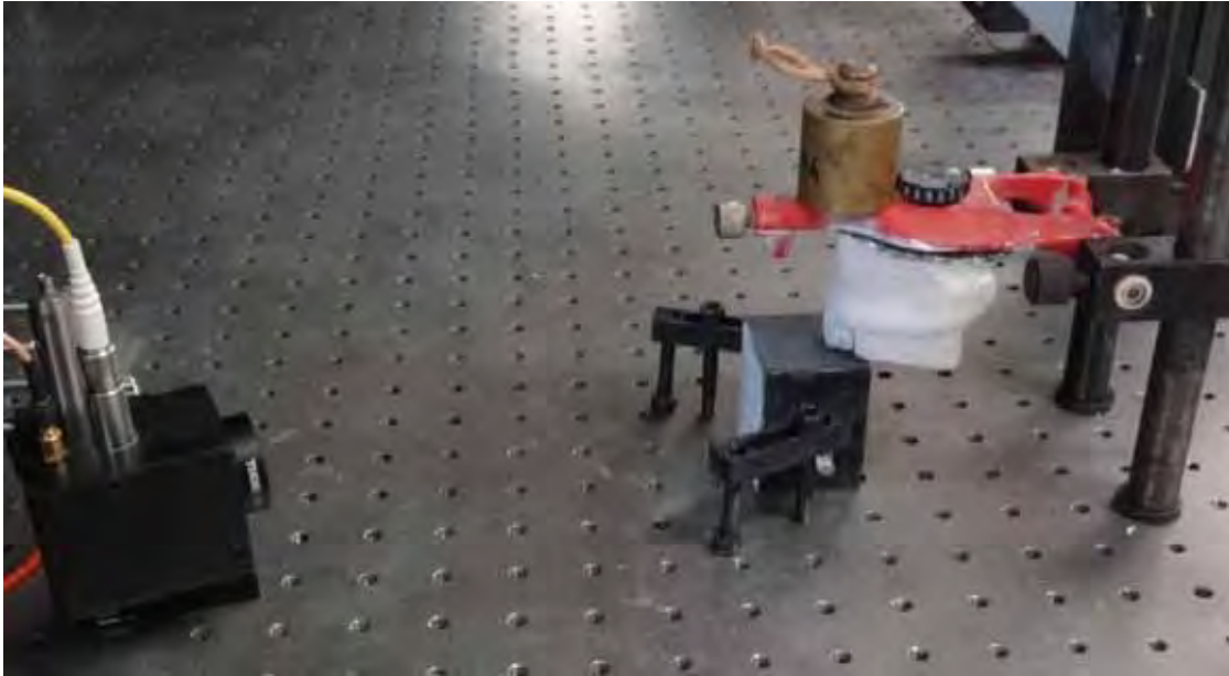
Figure 3 - Loading rig obtained for the ESPI measurements.
