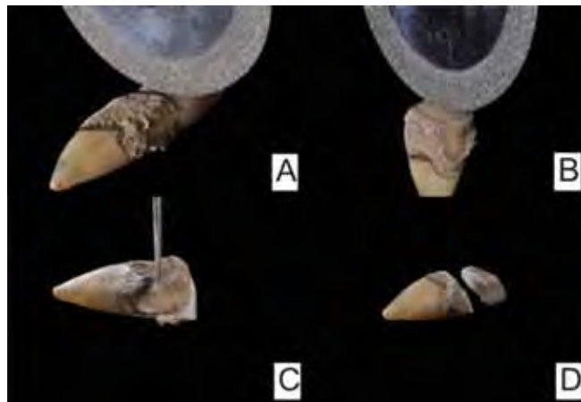
Figure 2 - A) Cutting with diamond disc separating the crown from the ROI. B) Cut in buccal-lingual orientation. C) Cutting in mesio-distal orientation. D) Separate sample.
