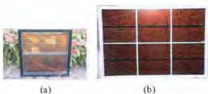
Fig. 1 (a) Transparent dye-sensitized solar cells (240 mm × 240 mm). (b) A unit module composed of 12 DSCs and a reflector of rugged aluminum plates (515 mm × 773 mm).
