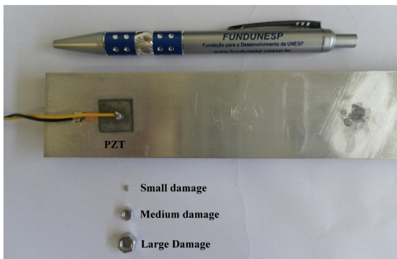
Figure 3. Aluminum beam with the PZT patch and damage of different intensities.
