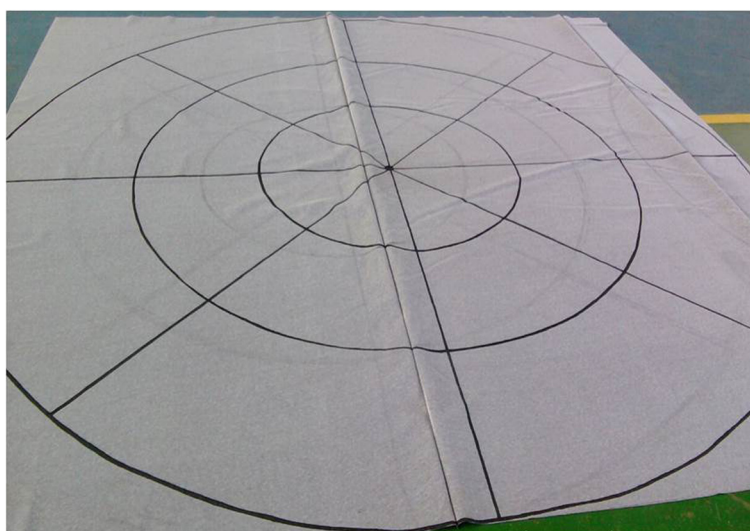
Figure 1 “Carpet” developed by researchers to evaluate the rotation and displacement of the patients.
