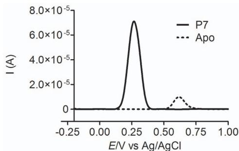
**Figure 10. Differential pulse voltammograms of 0.1 mM solutions of heptyl protocatechuate and apocynin at pH 7.0.** Differential pulse voltammograms were obtained at modulation time 0.05 s, pulse amplitude 0.05 V, step potential 0.45 mV and scan rate 4.5 mV/s. doi:10.1371/journal.pone.0110277.g010
