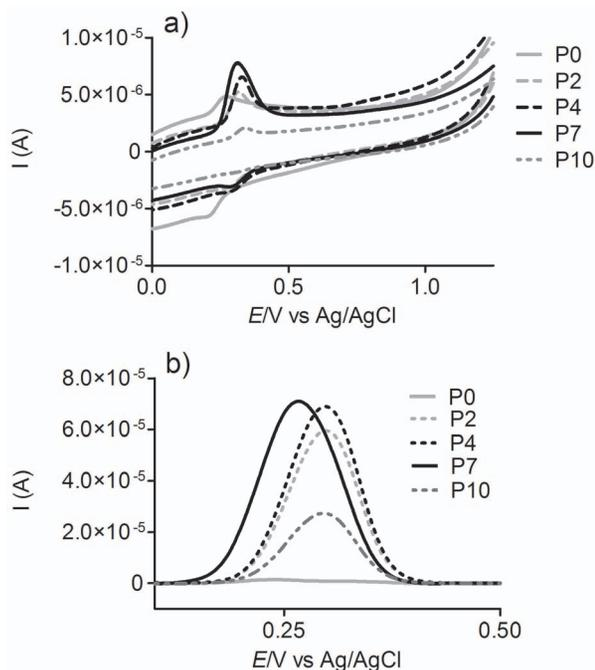
**Figure 9. Cyclic (a) and differential pulse voltammograms (b) of 0.1 mM solutions of protocatechuic acid and its esters at pH 7.0.** The cyclic voltammograms were recorded at a potential scan rate of  $5 \text{ mV s}^{-1}$ . Differential pulse voltammograms were obtained at modulation time 0.05 s, pulse amplitude 0.05 V, step potential 0.45 mV and scan rate 4.5 mV/s. doi:10.1371/journal.pone.0110277.g009
