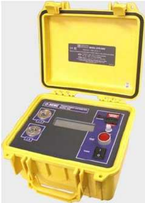
Figura 12 – TTR – Transformer Turn Ratio .
