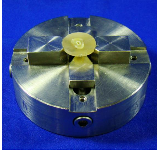
Figure 1: Metallic dispositive used to hold the samples during root canal enlargement and push-out test.
