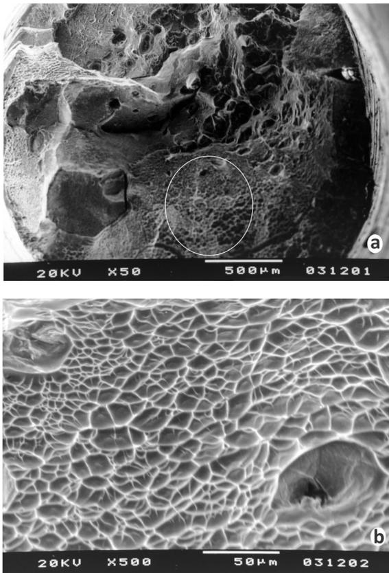
**Figure 3.** SEM images of sample A (a) 50x and (b) 500x regarding the circle, showing the dimples presence, after mechanical cycling test and tensile test.
