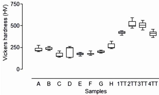
**Figure 2.** Distribution of Vickers hardness values (HV) for 12 distinct samples after mechanical cycling test (A-H) and heat treatment (1TT-4TT). The variance analysis result was significant ( $P < 0.0001$ ). Comparing 2 x 2 by Tuckey test, the results were statistically different ( $P < 0.001$ ) for all samples.
