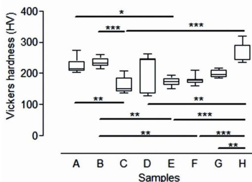
**Figure 1.** Distribution of Vickers hardness values (HV) for 8 distinct samples (A-H) after the mechanical cycling test. The variance analysis result was significant ( $P < 0.0001$ ). Comparing 2 x 2 by Tuckey test, the statistical results can be observed in the figure (\* =  $P < 0.05$ ; \*\* =  $P < 0.01$ , \*\*\* =  $P < 0.001$ ).
