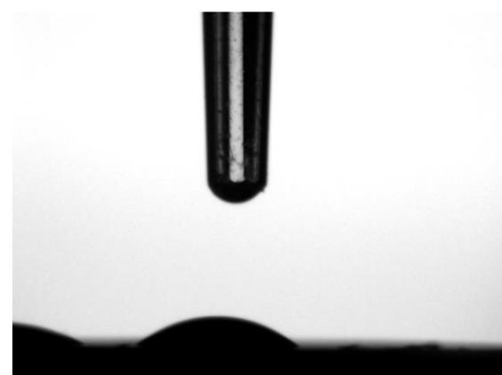
**Figure 3.** Contact angle values of the Ti specimens after electrochemical anodization treatment
