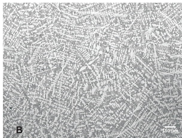
FIGURA 1 - Microstructures of Ni-Cr (A) and Ni-Cr-Ti alloys (B)
