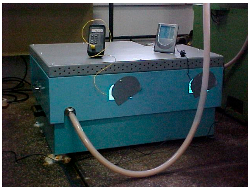
Figure 3. Side view of the reservoir with observation windows and inspection.
