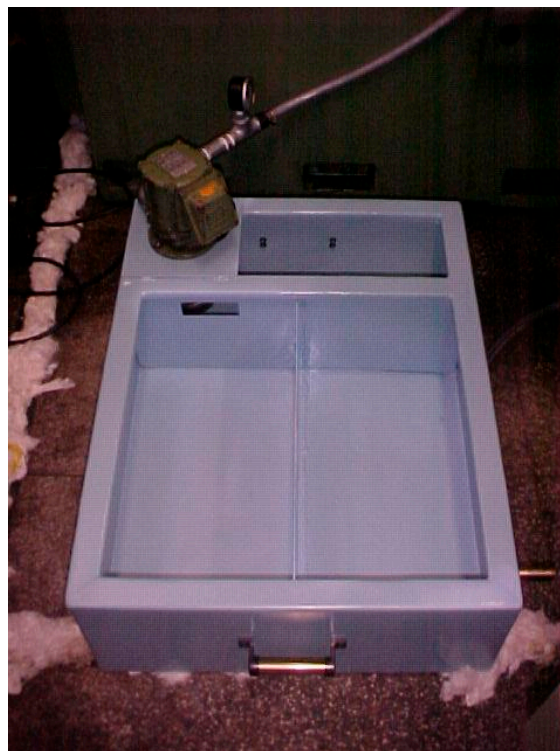
Figure 1. Top view of the shell with three compartments and suction pump.
