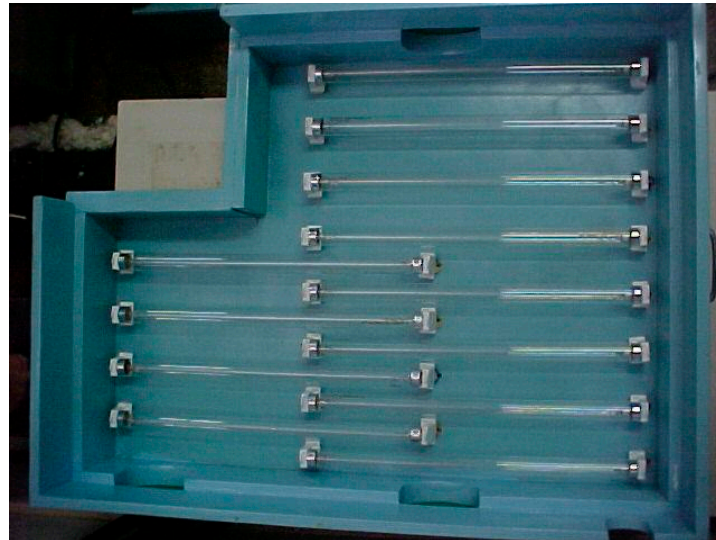
Figure 2. Inside view of the ultraviolet radiation emitter system and layout of the germicidal lamps.
