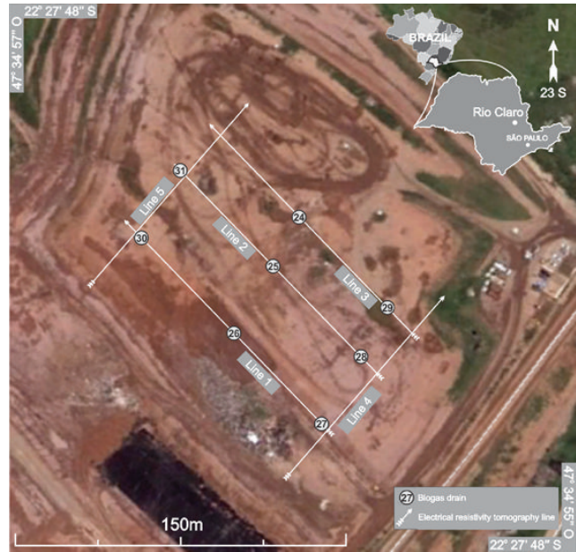
FIGURE 1: Location of the area of studies with position of the lines of data acquisition and drains for measuring the flow of biogas.
