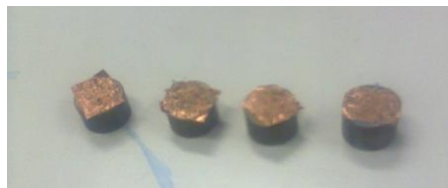
Figure 1. Specimen holder with the double-sided copper tape and sugarcane samples (1.0 mm particle size)
