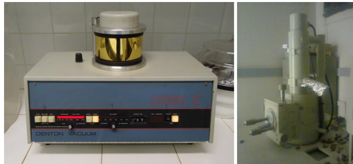
Figure 2. Machine (JEOL JFC 1100) on the left and scanning electron microscope on the right (JSM5410).
