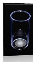
Desgaste 50 µm Lixa 400 (CARBIMET – BUEHLER)
