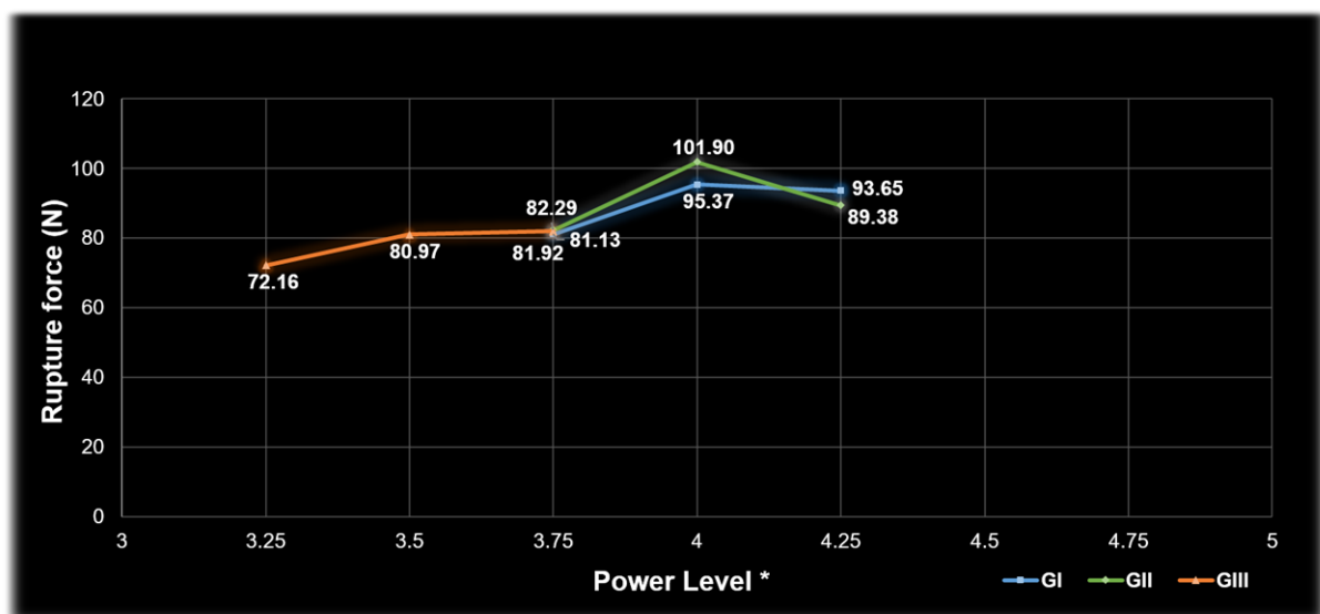
Figure 2 Graph of the maximum force registered before rupture given the power levels used for welding of the three groups tested. *Each power level is equivalent to 500W.
