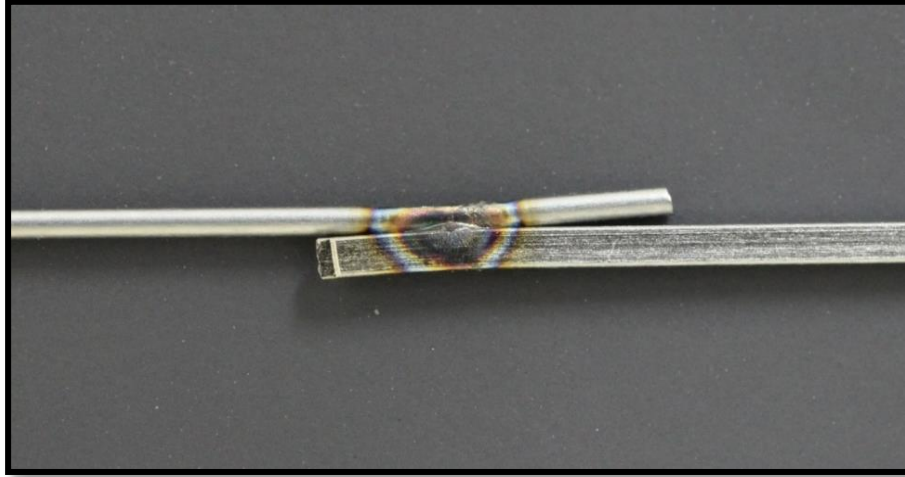
Figure 1 Spot electric welding of NiTi wires (0.018" and 0.017" x 0.025").
