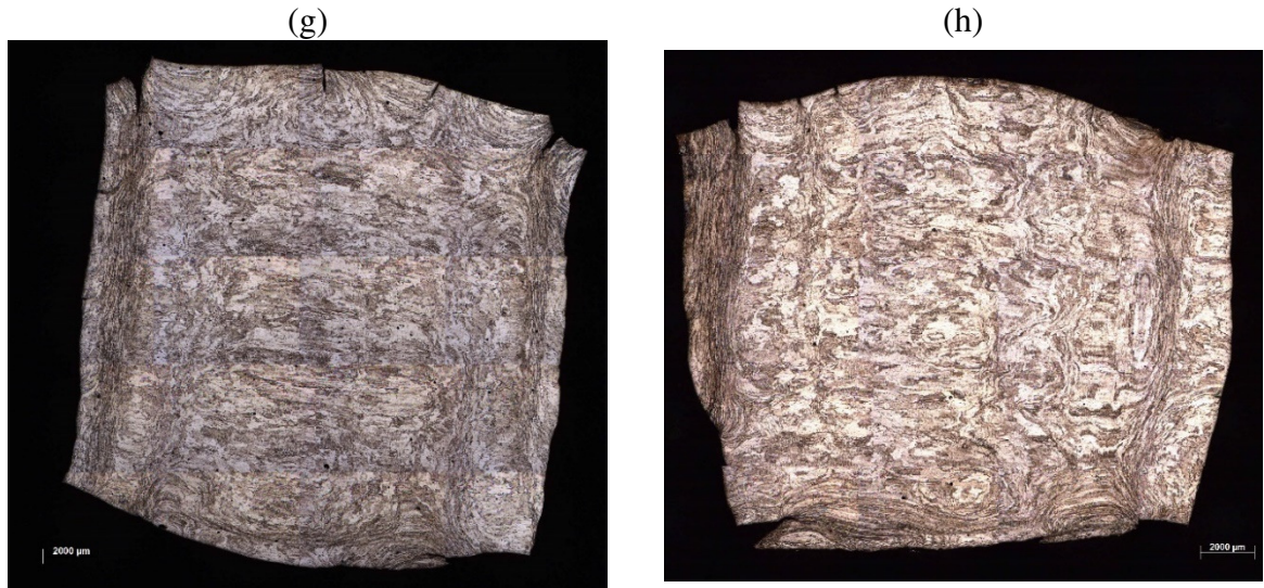
Figura 40 – Macroscopia das amostras atacadas com reagente Keller: (a) #1 (0%); (b) #2 (26%); (c) #3 (39%); (d) #4 (43%); (e) #5 (50%); (f) #6 (57%); (g) #7 (59%); (h) #8 (64%). (conclui)
