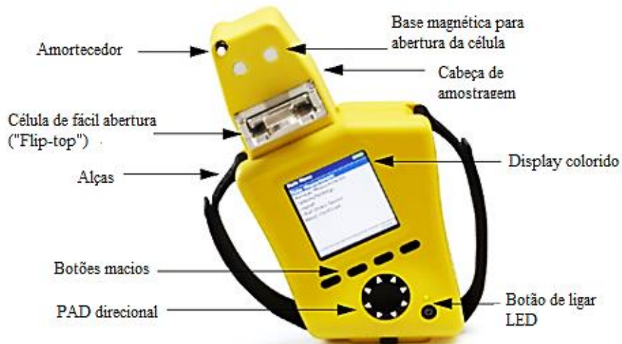
Figura 25 – Detalhes do Fluid Scan Q1000
