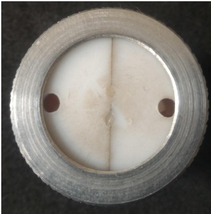
Figure 3. Teflon matrix and metallic ring used to built-up the composite resin cylinders.
