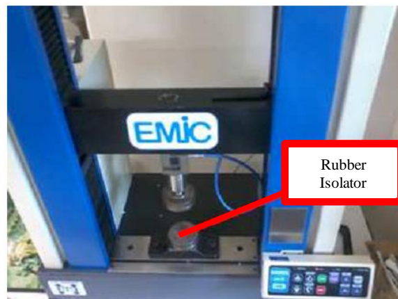
Figure 30 – Measurement scheme to determine the static properties.
