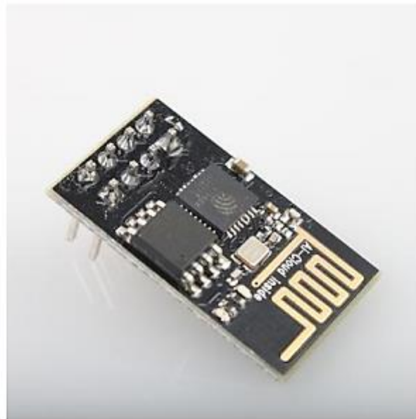
Figure 3 [Module Pin Counts, 8 pin, 14.3 mm *24.8 mm *3.0 mm]
