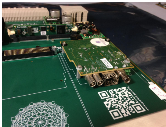
Figure 12 - TTC FMC attached to the Pulsar 2b board.
