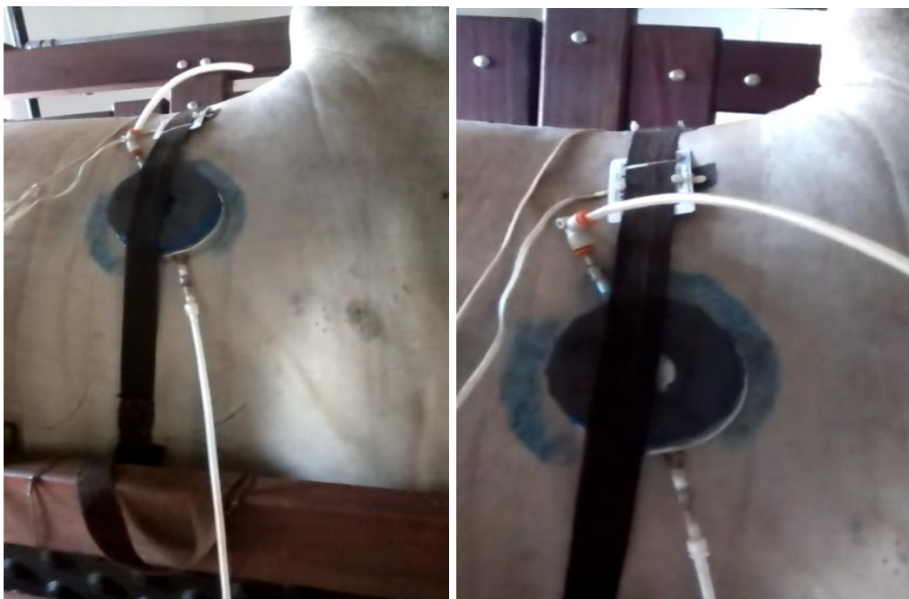
Figure 4: Ventilated capsule under the unshaved cutaneous surface area of the Nellore cattle.
