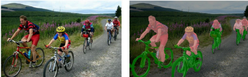
Figure 9: Semantic parser of image. In the left, the original image. In the right, bikes and people detect by using this technique
