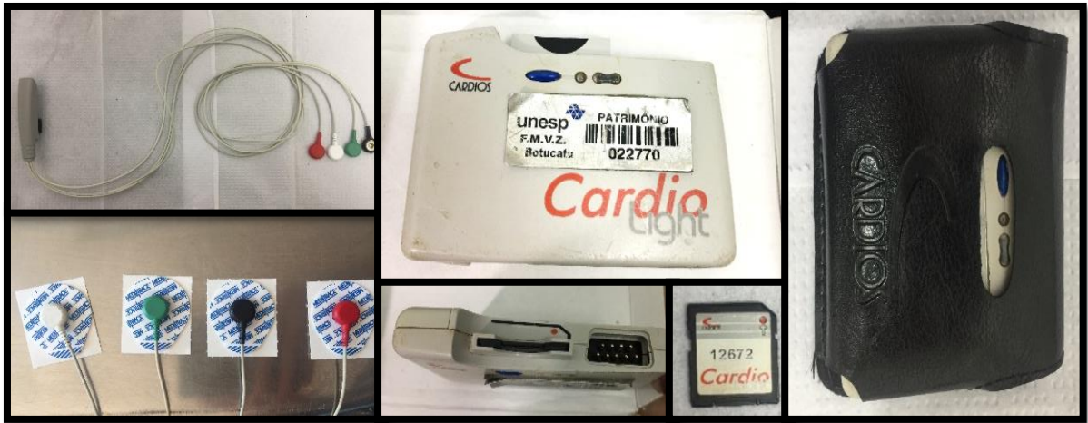
Figure 4. Holter Equipment – Cables, electrodes, SD Card and protective cover.
