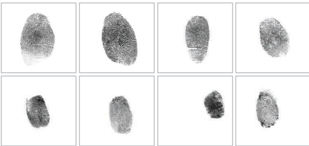
Figure 1. Fingerprints from the Crossmatch 2013 [4] dataset. The top fingerprints are real and the bottom are fake, i.e., obtained from synthetic fingers made of different materials.
