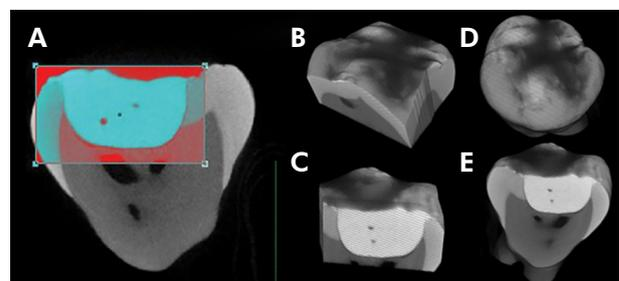
**Figure 1.** 3D reconstruction of cavity filled with resin composites. Illustrative 2D slice showing the region of interest - ROI (Figure A - red square). Restoration at different angles (B, C, D, and E).
