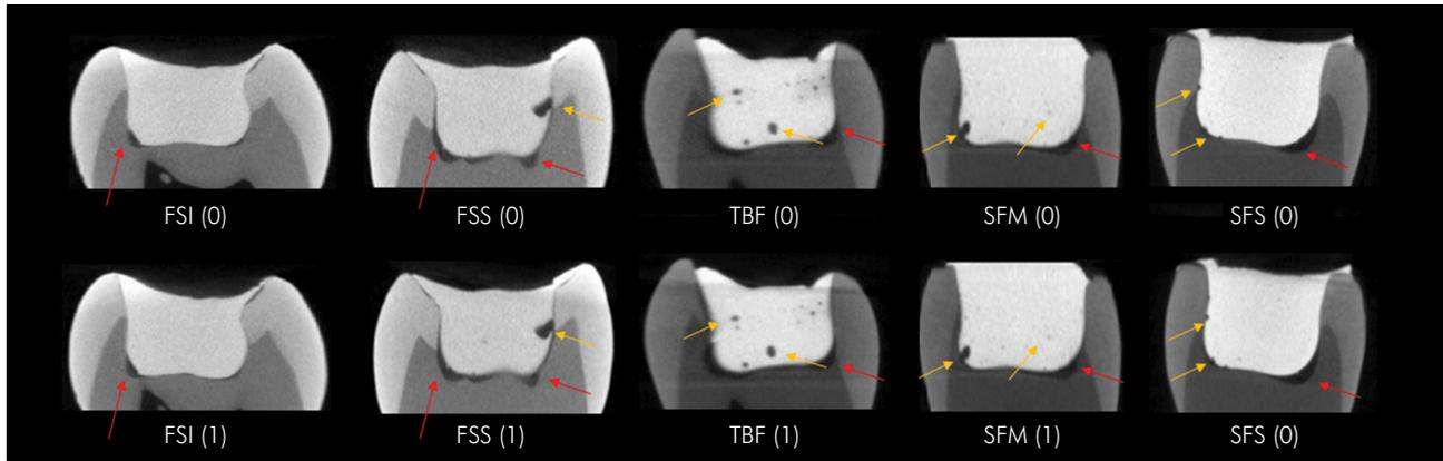
**Figure 3.** Presence of gaps and voids in the resins before (0) and after (1) light curing indicated by arrows in the  $\mu$ CT (red=gap; yellow=void). FSI: Filtek Supreme XTE - incremental insertion; FSS: Filtek Supreme XTE - single insertion; TBF: Tetric Bulk Fill; SFM: SonicFill - manual filling; SFS: SonicFill - sonic filling.
