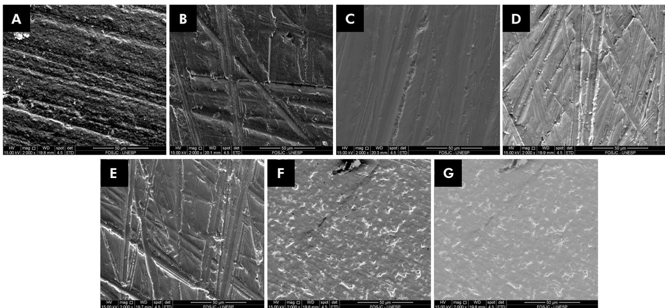
**Figure 1.** Scanning electron microscopy (2,000x magnification) of surface patterns in each group. Control (Top, center); G80 (1<sup>st</sup> row, left column); G80A (1<sup>st</sup> row, right column); G120 (2<sup>nd</sup> row, left column); G120A (2<sup>nd</sup> row, right column); G600 (3<sup>rd</sup> row, left column); G600A (3<sup>rd</sup> row, right column).
