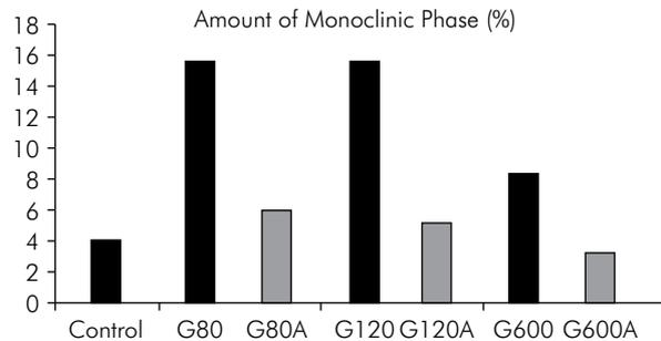
**Figure 2.** Relative amount of monoclinic phase, according to X-ray diffraction analysis in each tested group: CG (4.15%), G80 (15.64%), G80A (5.97%), G120 (15.6%), G120A (5.24%), G600 (8.39%), G600A (3.27%).
