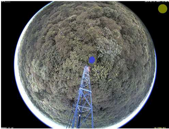
Fig. 19. Example of daily vegetation image taken in the context of e-phenology project, and the mask (blue shadow) for a species crown, that represents a region of interest (ROI). Based on the processing of the ROI within the image, we can extract some temporal features for the vegetation, for instance, the green chromatic correlation G_{cc} variation (Alberton et al., 2017; Alberton et al., 2014).
