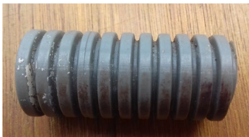
Figure 4 Corrugated PVC rings with 400 mm length, 190 mm internal diameter, specific surface area of 135 \text{ m}^2/\text{m}^3 and 87% of void volume.
