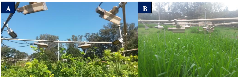
Figure 3. Temperature Free-Air Controlled Enhancement (T-FACE) system in S. capitata (A) and P. maximum (B). Photos by Carlos Martínez y Huamán.
