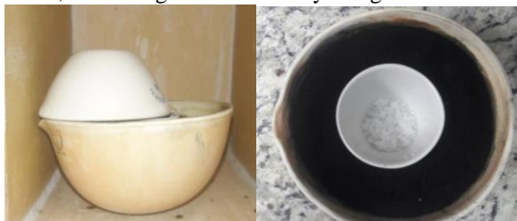
Figure 3.1 Scheme of the SiO_2:Ba^{2+}, Tb^{3+} xerogel calcination by using charcoal as an in situ source for CO.
