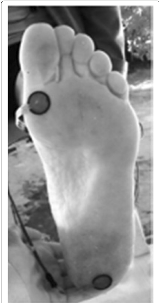
Fig. 1 Positioning of pressure sensors for gait analysis
