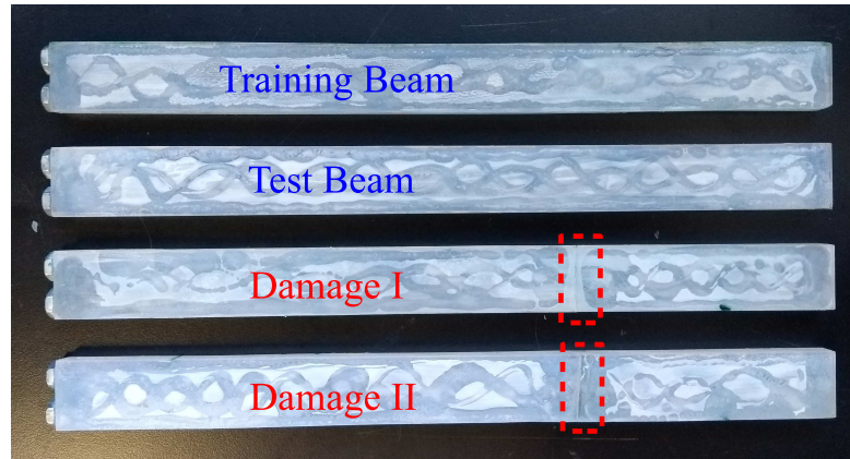
(a) All beams constructed.
