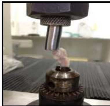
Figure 3. Mechanical compression test on the femoral head.
