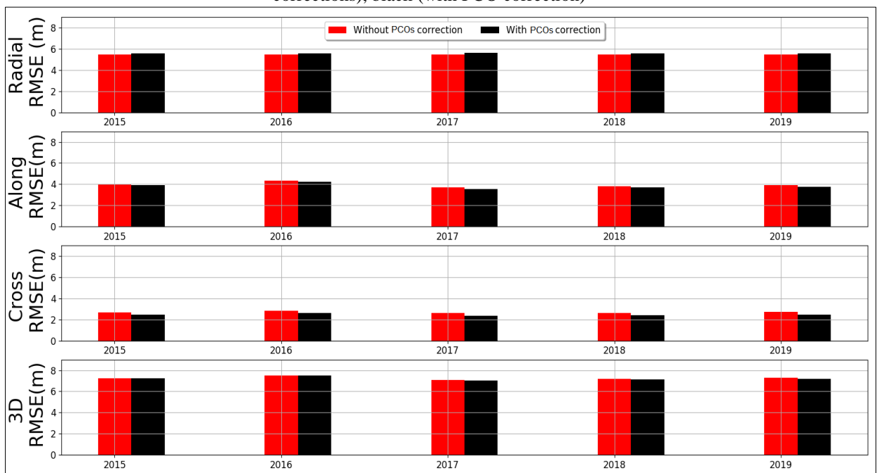
Figure 18 - RMSE for the Radial, Along-track, Cross-track, and 3D by year for GLONASS. Red (without PCO corrections), black (with PCO correction)
