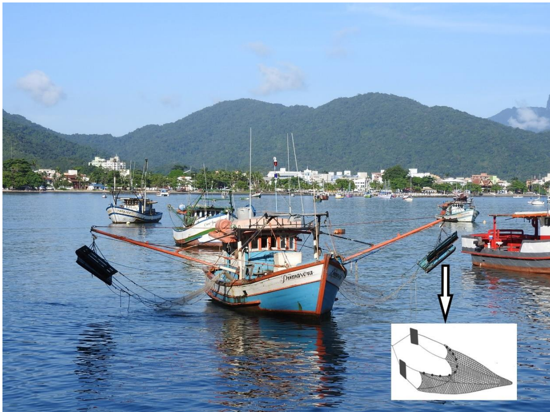
Figure 2. Shrimp trawling fishing boat. Fishing boat equipped with two double rig nets. The two nets are identical and during the trawling these are used simultaneous. Detail of the illustration of the doors positioned inside the water.
