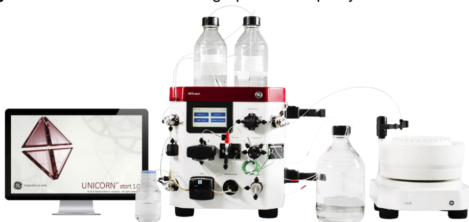
Figure 4 - AKTA Start chromatograph used to purify 5'-ribonucleotides.
