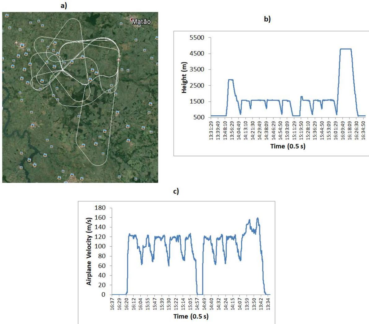
**Figure 2:** Path of airplane (a), Geometric height (b) and velocity (c) for flight 811.
