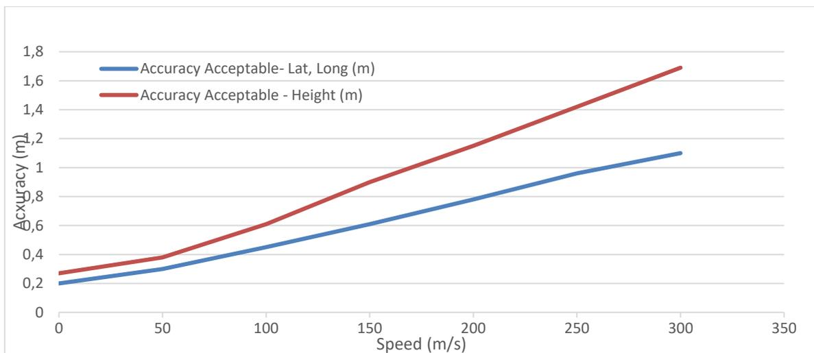
**Figure 1:** Required accuracy for aircraft flight tests.
