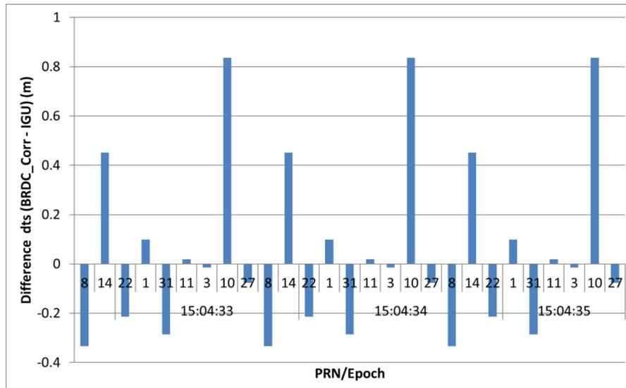
**Figure 11:** Discrepancies for satellite clocks from IGU and broadcasted with corrections (BRDC+Corr).
