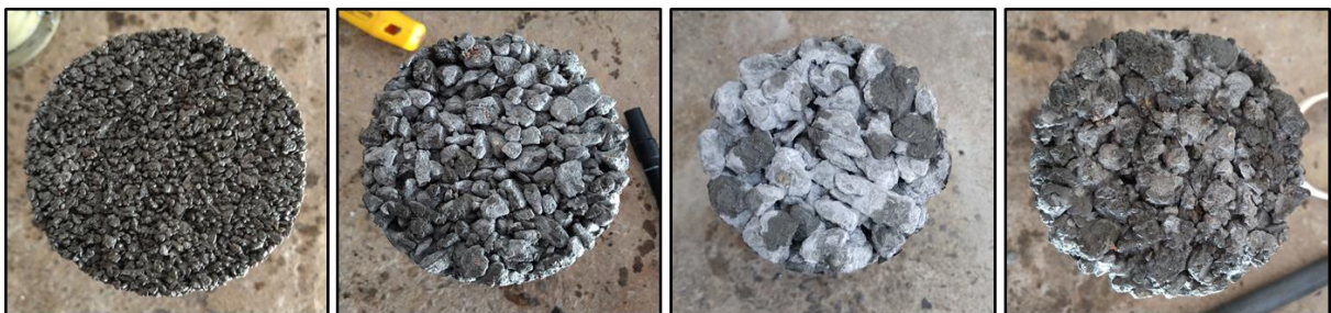
Figure 2.7 - Visual comparison of pervious concrete samples with aggregates of different dimensions and combinations
