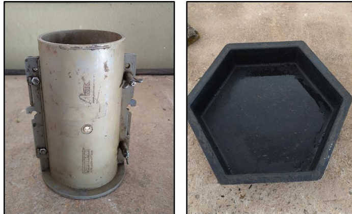
Figure 3.4 - Cylindrical and hexagonal molds for making pervious concrete mold
