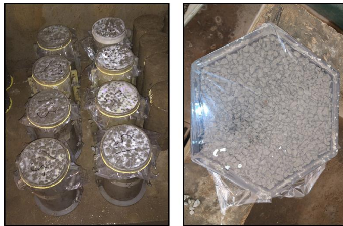
Figure 3.6 - Newly molded and plastic-covered specimens
