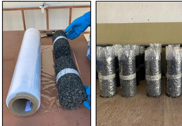
Figure 2.9 - Preparation of samples for infiltration rate testing according to ISO 17785-1
