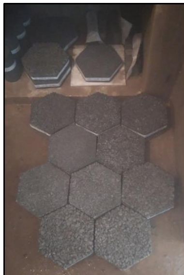
Figure 3.7 - Samples placed in a humid chamber for 28 days
