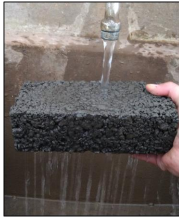
Figure 2.2 - Pervious concrete percolating water
